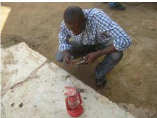
**Stephen cleaning antenna parts with kerosene from a lantern. With nowhere to buy new hardware, all rust was removed from nuts, screws and bolts using files and brushes**
