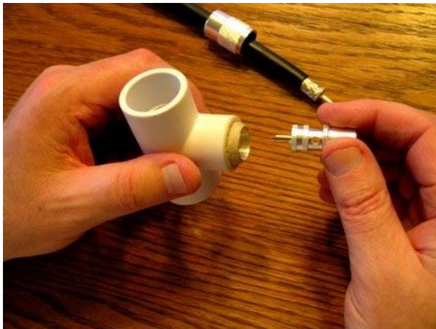
Prep the coax as usual, but then thread the PL-259 connector into the new tool.
